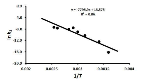
Figure 3: Arrhenius plot  $Ln(k_1)$  versus 1/T
