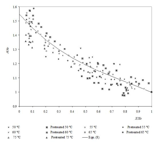
Figure 3: Relative surface area  $(A/A_o)$  of particles as a function of the relative water content  $(X/X_o)$  for pretreated and not pretreated whole rose hip fruits at various drying air temperatures. The solid line represents model-predicted values by Eq. (11)
