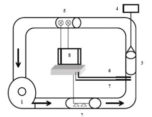
Figure 1: Scheme of the experimental equipment employed in this work 1. Variable speed fan. 2. Relative humidity conditioner, with saturated salt solutions. 3. Removable drying chamber. 4. Balance. 5. PC-controlled electric heater, using a purpose-developed Visual Basic Program 6. Data logger for dry bulb temperature of air. 7. Relative humidity meter. 8. Personal Computer (PC).
