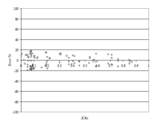
Figure 5: Percentage errors of model-predicted values of  $V/V_o$  by Eq. (12) as a function of the experimental  $X/X_o$  for the three fruits.
